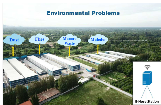
Fig. 1. Environmental problems of poultry farm and E-nose station for odor monitoring
