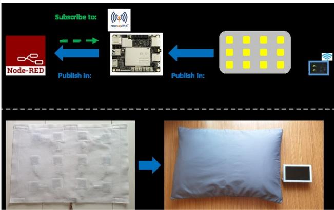
Fig. 2. Architecture of non-obstructive monitoring system for human's sleep monitoring.
