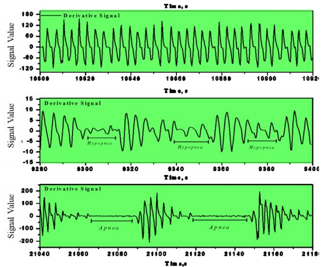
Fig. 4. Comparison of sleep signal from the data pillow for normal respiration, hypopnea and apnea.
