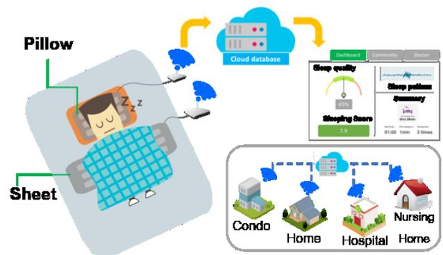
Fig. 1. The concept of non-obstructive monitoring system for human's sleep monitoring.
