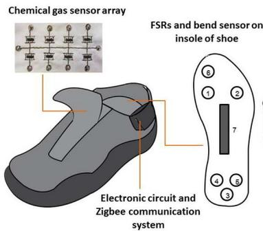
Fig. 2. Various sensors installed inside the healthcare shoe.
