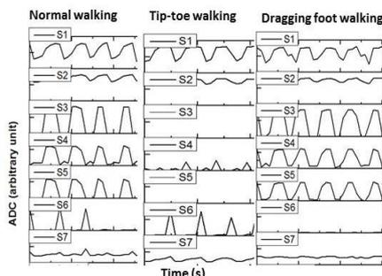
Fig. 3. Typical signals obtained from FSRs (no. S1-S6) and bend sensor (no. S7).
