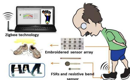
Fig. 1. Schematic diagram of healthcare shoe monitoring system
